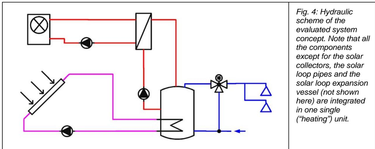
*Fig. 4: Hydraulic scheme of the evaluated system concept. Note that all the components except for the solar collectors, the solar loop pipes and the solar loop expansion vessel (not shown here) are integrated in one single ("heating") unit.*
