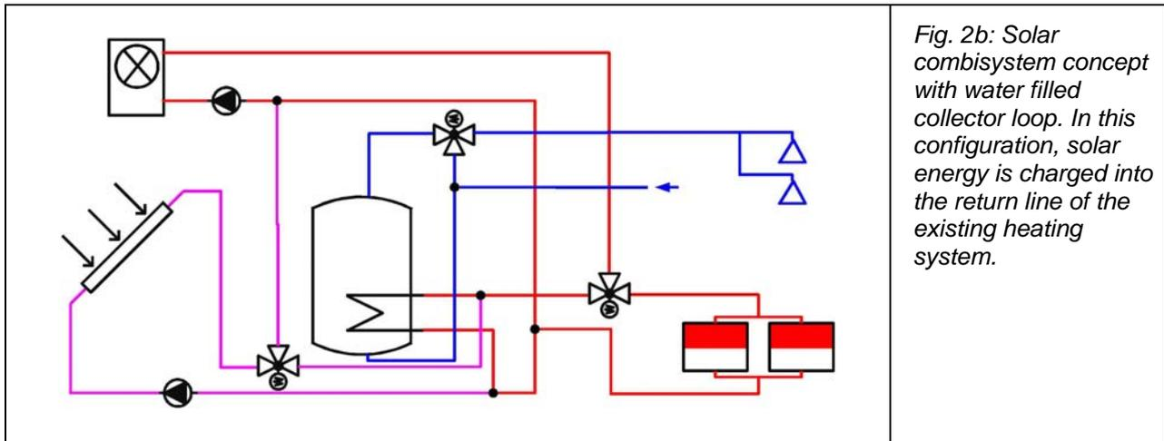
*Fig. 2b: Solar combisystem concept with water filled collector loop. In this configuration, solar energy is charged into the return line of the existing heating system.*
