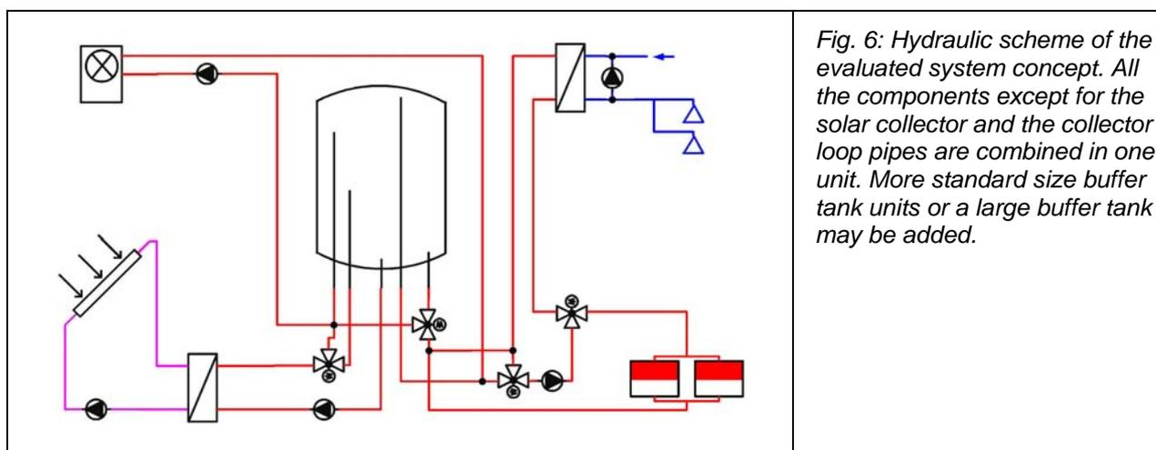
Fig. 6: Hydraulic scheme of the evaluated system concept. All the components except for the solar collector and the collector loop pipes are combined in one unit. More standard size buffer tank units or a large buffer tank may be added.
