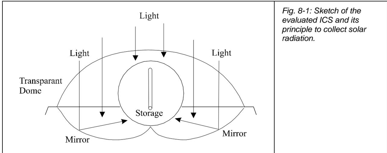
*Fig. 8-1: Sketch of the evaluated ICS and its principle to collect solar radiation.*
