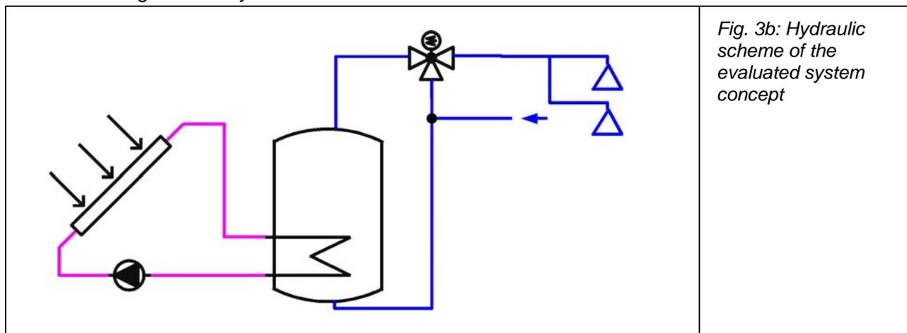
Fig. 3b: Hydraulic scheme of the evaluated system concept
