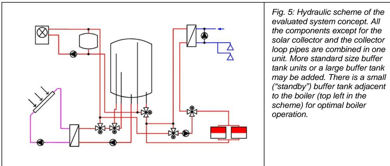
*Fig. 5: Hydraulic scheme of the evaluated system concept. All the components except for the solar collector and the collector loop pipes are combined in one unit. More standard size buffer tank units or a large buffer tank may be added. There is a small (“standby”) buffer tank adjacent to the boiler (top left in the scheme) for optimal boiler operation.*
