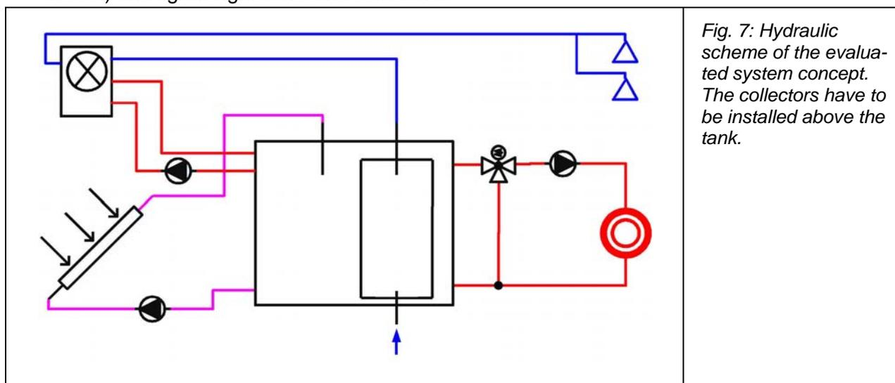
*Fig. 7: Hydraulic scheme of the evaluated system concept. The collectors have to be installed above the tank.*
