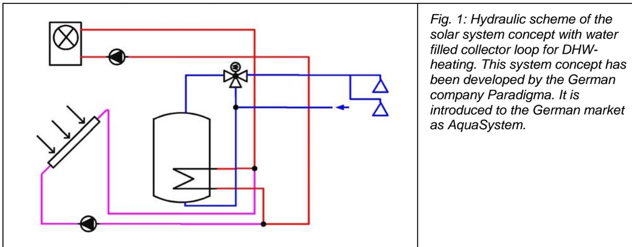
*Fig. 1: Hydraulic scheme of the solar system concept with water filled collector loop for DHW-heating. This system concept has been developed by the German company Paradigma. It is introduced to the German market as AquaSystem.*
