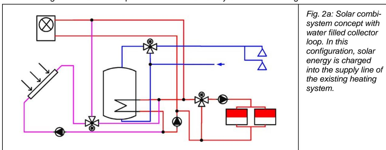
*Fig. 2a: Solar combi-system concept with water filled collector loop. In this configuration, solar energy is charged into the supply line of the existing heating system.*
