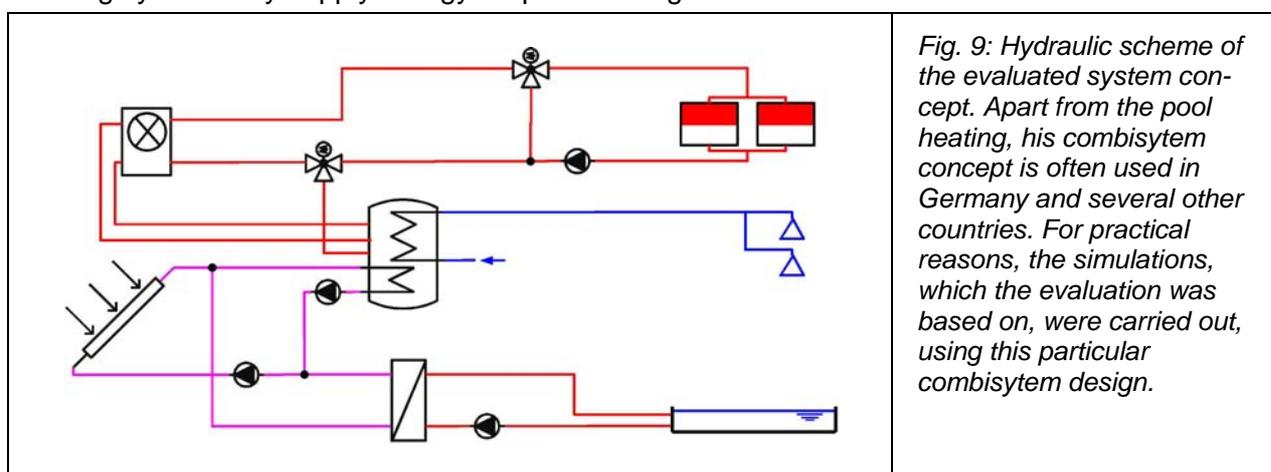
*Fig. 9: Hydraulic scheme of the evaluated system concept. Apart from the pool heating, this combisystem concept is often used in Germany and several other countries. For practical reasons, the simulations, which the evaluation was based on, were carried out, using this particular combisystem design.*
