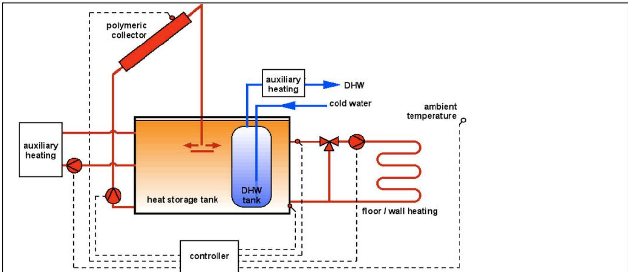
2a) Hydraulic scheme of a solar heating system with drain-back design and polymeric collectors.
