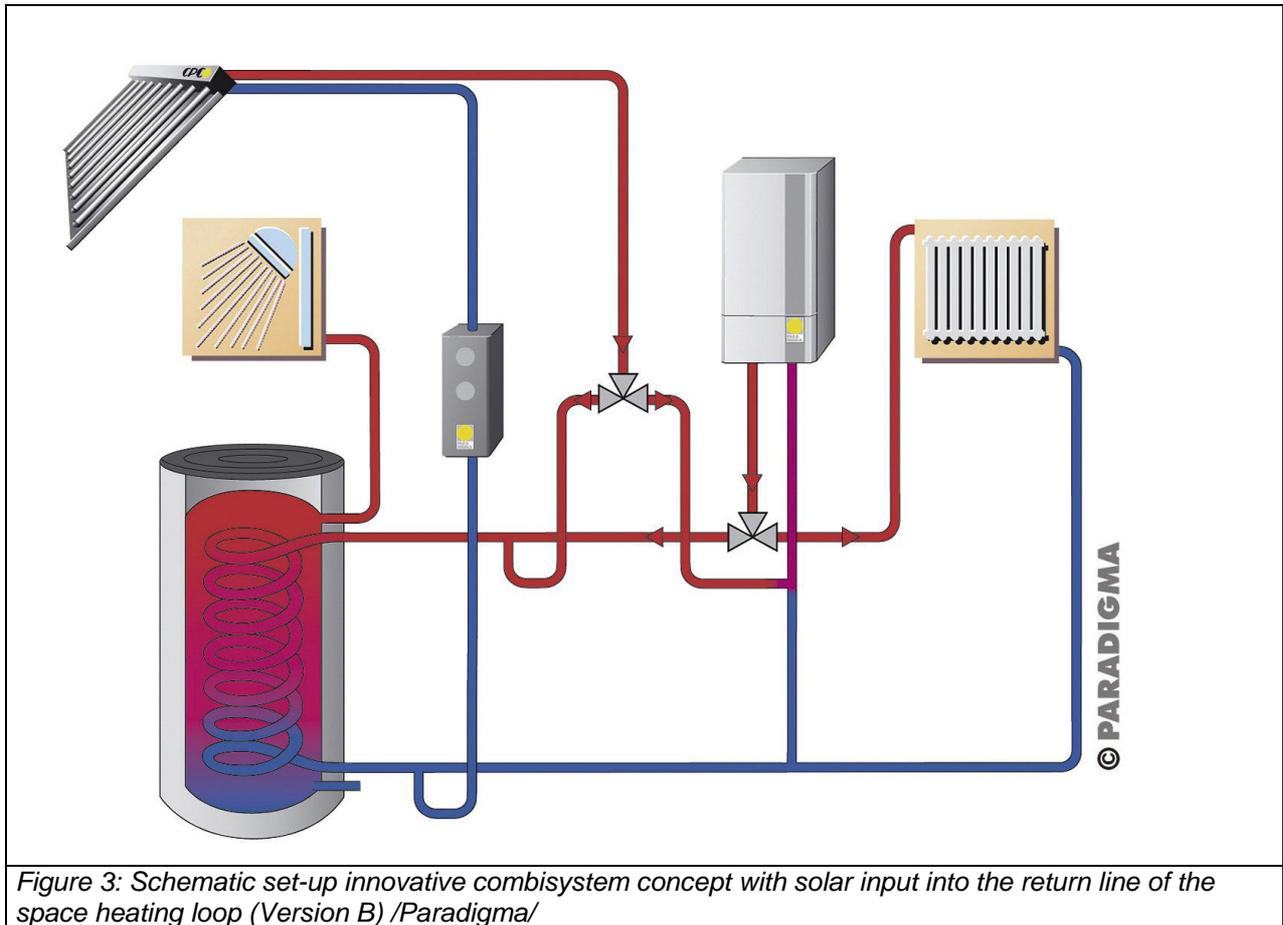
Figure 3: Schematic set-up innovative combisystem concept with solar input into the return line of the space heating loop (Version B) /Paradigma/
