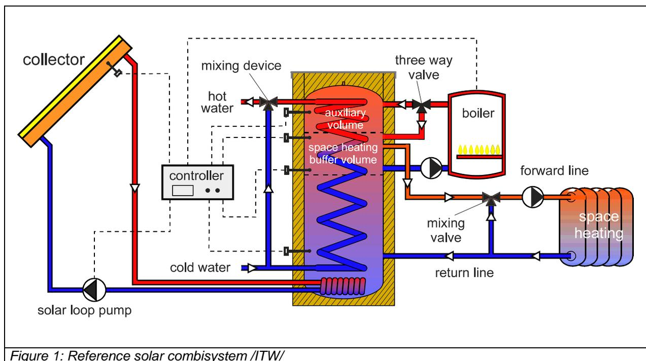
Figure 1: Reference solar combisystem /ITW/
