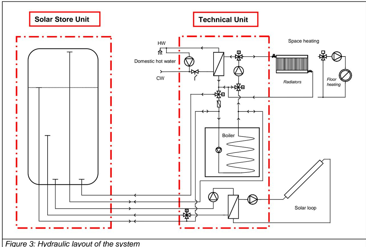
Figure 3: Hydraulic layout of the system
