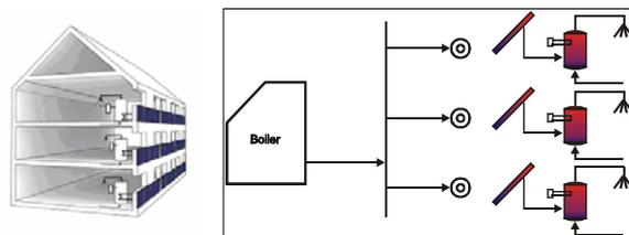
Figure 4: Decentralized Solar Thermal System
