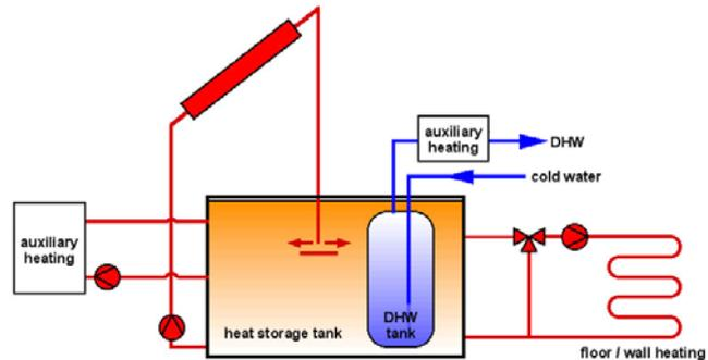
Figure 3: Non-pressurized Drain-Back System
