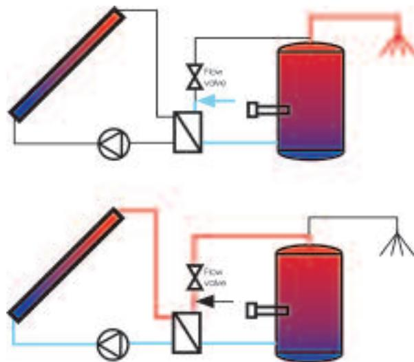
Example with solar collector connected via heat transfer unit with special back flushing configuration for anti-fouling ENERWORKS
