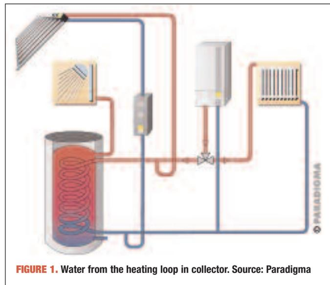
FIGURE 1. Water from the heating loop in collector. Source: Paradigma
